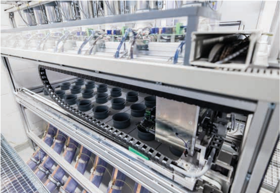
Thanks to modern motor technology, transport carriers are transferred precisely and reliably between different zones. Smooth-running, high-precision, and durable guidance systems ensure maximum reliability and long-lasting product quality.
